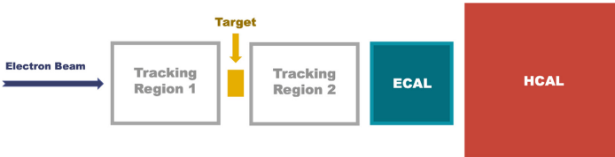
Fig. 2. The detector scheme for the beam-dump experiments in this study. There are two tracking regions for reconstructing track of the incident electron and its products after interacting with the nuclei in the target. ECAL and HCAL are behind the tracking region.
